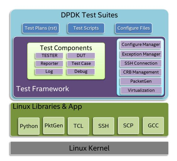
DPDK Test Suite environment includes DUT (Device under Test), Tester and packet generator. DPDK software will deployed and run on DUT. DPDK Test Suite should run on the Tester.
