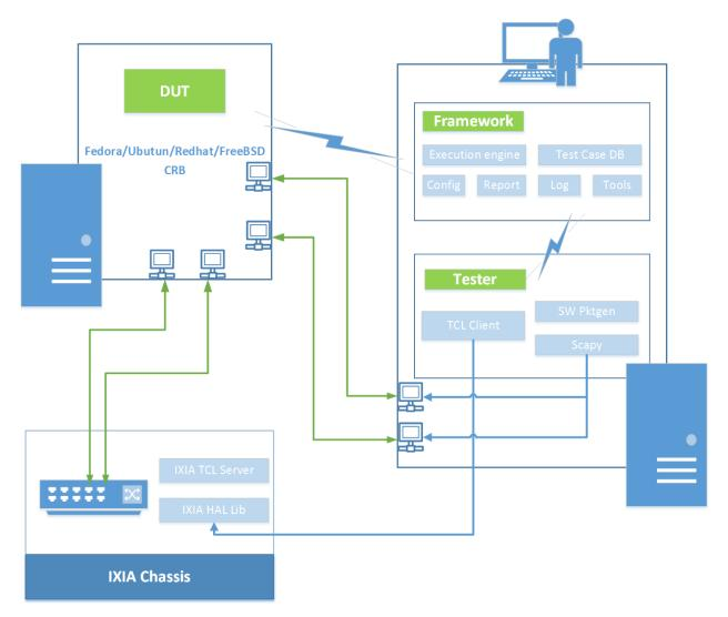
This architecture provides automatically mechanism to manage tester, DUT and packet generators, and remove dependency between test script and test environment/hardware. It defines one abstraction layer for DPDK Test Suite, and provides extensibility to add more test script. In the DPDK Test Suite Test Framework, it provides the following modules to help to manage device, platform, configure and test results.
